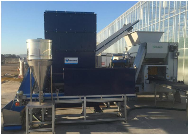
The Logitec CM 200 can be supplied in various configurations. From a simple manual system to fully automatic. An optional touch screen control panel will allow for perfect moisture control and the possibility for recipe building. Coir blocks are filled automatically into the Coir Mill using a special pallet lift.
