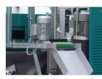
The TM 2400 E is compatible with all popular automation and transplanting systems and has a flexible arrangement of the conveyor belt at 8 positions around the turntable.
