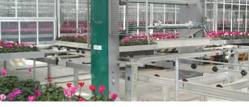
With this system, efficiency and precision go hand in hand. The TR 4103 is a quiet operation that effectively displays both power and accuracy as it places pots on mobile benches, trailers or collating conveyors (PLC-controlled). As an automatic distribution center, it offers improved processing potential, ideally suited to powerful, large volume potting machines. With its durable 5.7" touch screen it is easy to program and input data.
