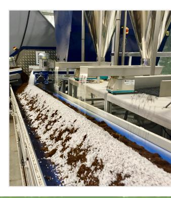
The Logitec Plus Mixing Lines can process a wide variety of products including: White and Black peat, Compost, Sand, Clay, Perlite, Vermiculite, Osmocote, Lime, Both Artificial and Organic Fertilizers.
